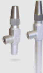
The stainless steel needle valves (SNV-SS) are compact and light service valves. They are especially suited for heavy-duty industrial applications due to their sturdy design and high level of operating safety. Their design provide a high flow characteristic. The SNV-SS valves have a maximum operating pressure of 52 bar in the pressure range of -60 °C to +150 °C.
