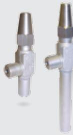
The stainless steel needle valves (SNV-SS) are compact and light service valves. They are especially suited for heavy-duty industrial applications due to their sturdy design and high level of operating safety. Their design provide a high flow characteristic. The SNV-SS valves have a maximum operating pressure of 52 bar in the pressure range of -60 °C to +150 °C.
