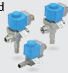
EVRS and EVRST stainless steel solenoid valves are based on three different principles: Direct, servo or forced servo operation. The forced servo operated valves, designed for keeping open at a pressure drop of 0 bar, can be used in liquid, suction, hot gas and oil return lines. EVRS and EVRST come equipped with a spindle for manual opening and have a working pressure of 50 bar and can handle media temperatures from -40 °C up to +105 °C (max temperature is dependent on coil).
